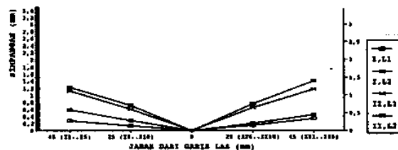
Gambar A18 Simpangan Distorsi Angular Flange Sambungan T (h = 6 mm, l = 150 A, v = 1,6 mm/detik)
