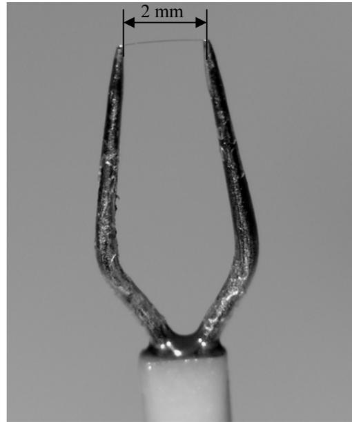
Gambar 1. Single normal hot-wire sensor
