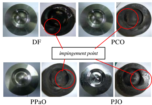
Figure 12. Piston Condition After Test Compare to New Condition
