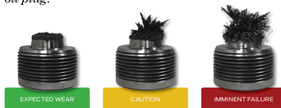
Gambar 7. Kondisi oil plug
