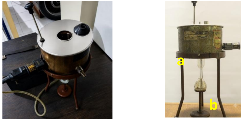
Figure 3. Viscometer used in this study: a) Upper reservoir, b) Lower reservoir
