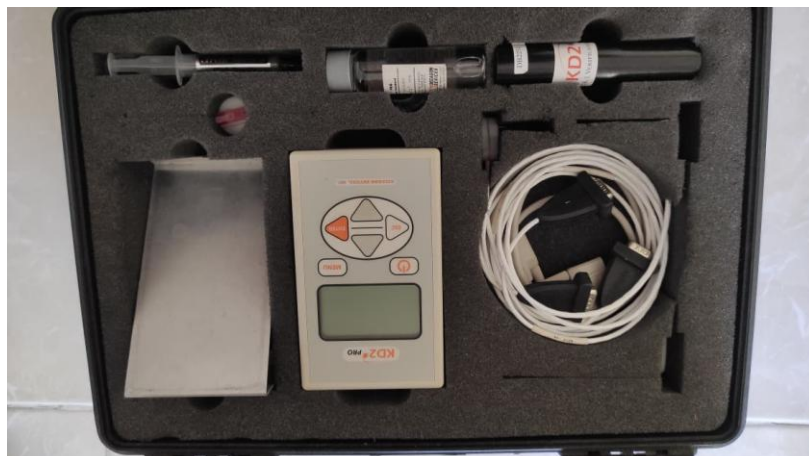
Figure 2. The KD2 Pro Analyser to measure the thermal conductivity of BCO
