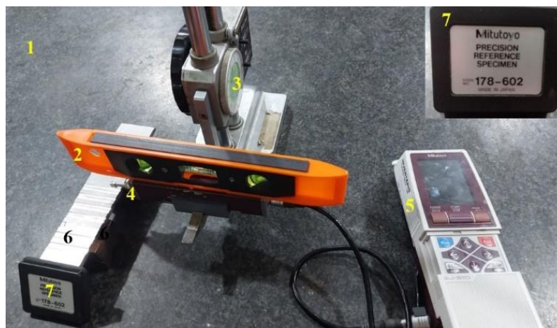
Figure 4. Equipment setup for surface roughness measurement: 1 – Wanzel Präzision measuring stand; 2 – Waterpass; 3 – Dial height gauge; 4 – Surface roughness sensor; 5 – Visual and communication device for surface roughness sensor; 6 – Workpiece; 7 – Calibrator
